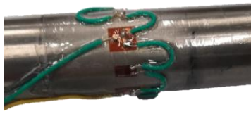
Figure 6 - Load cell installed in one of the transmitter bars.
